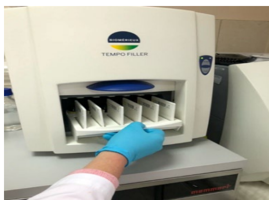
Fig. 4. TEMPO® Filler Sample Preparation Station (card filling and sealing)
